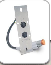
Take advantage of CPI's waterproof switches mounted in easy-to-install panels. Switches can be wired in series, parallel, or left as individual circuits. Panel assemblies can be terminated with a wide variety of industry standard connectors.
